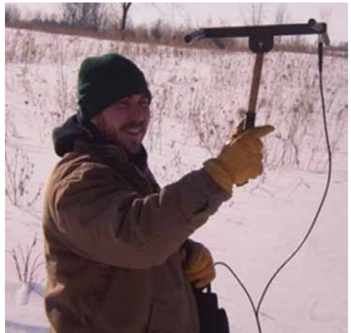
FIGURE 3. Undergraduate researcher using VHF telemetry to locate ring-necked pheasants in order to remotely download GPS spatial locations from a pheasant GPS collar.
